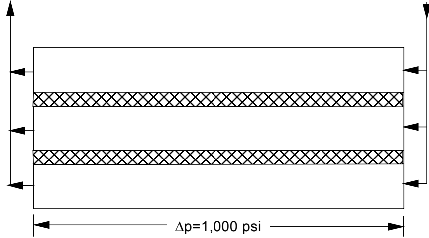
Fig. 7. Channeling model with no crossflow between adjacent layers.
