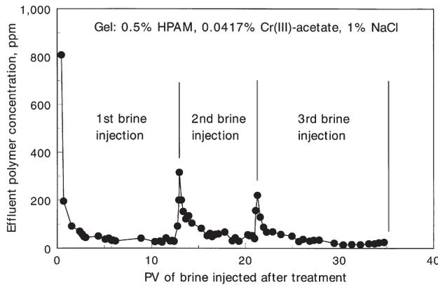
Fig. 3—Effluent polymer vs. PV of brine injected after treatment.
