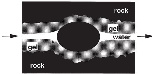
**Fig. 2—Balance between capillary forces and gel elasticity when forcing oil or water through an aqueous gel.**
