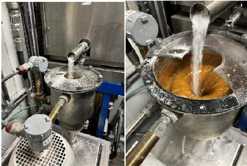
**Fig. 7—Corrosion due to lack of nitrogen blanket at the E-Pad.**
