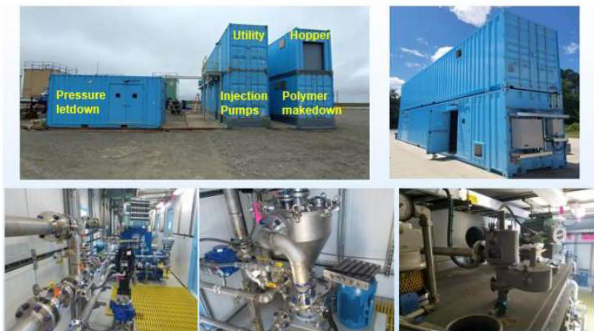
Fig. 11—Polymer makeup and injection skid for the J-Pad (Ning et al. 2019).
