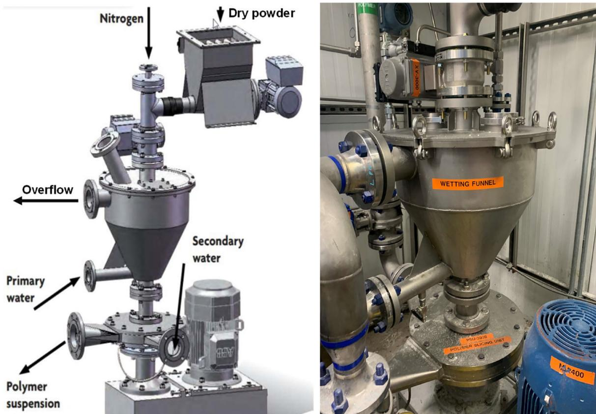
Fig. 13—Effective polymer slicing unit for polymer dissolution (schematic on the left; actual on the right).
