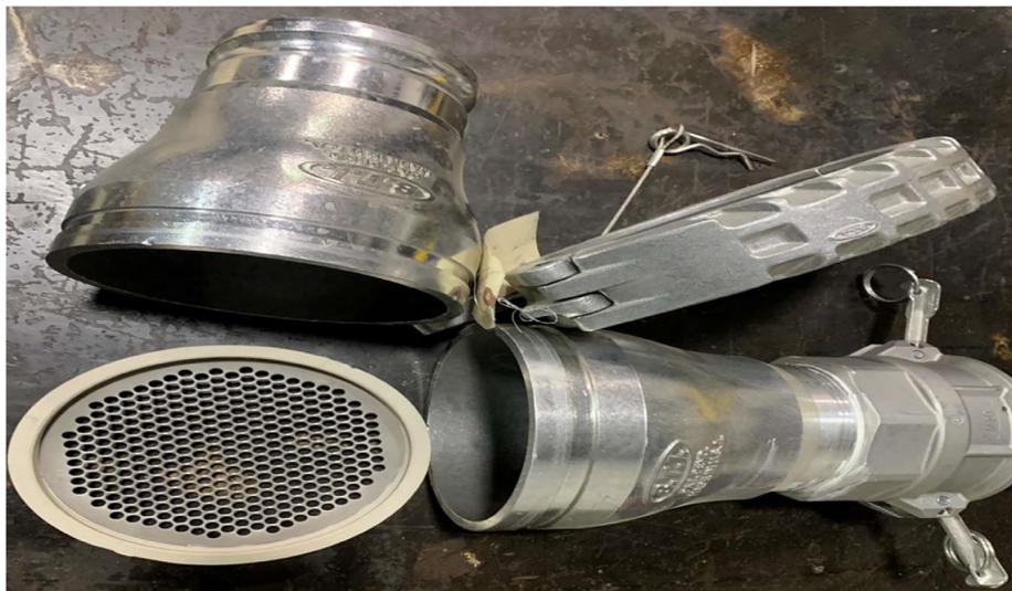
Fig. 12—Screen used during polymer transfer into a storage silo.
