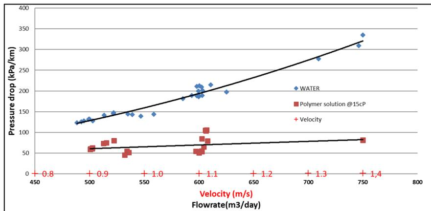
**Figure 8** Pressure drop of water and polymer solution (FP 3630S - 15cP @7,34s<sup>-1</sup>) versus flow rate and fluid velocities in a 4 inches diameter pipe over several kilometres.
