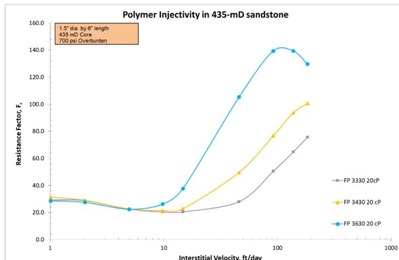
**Figure 6** In-situ rheology of 3 different polymers injected at the same viscosity. Flopaam 3330S, 3430S and 3630S (from medium to high molecular weight). The onset and amplitude of shear-thickening are earlier and higher for the high molecular weight product FP3630S compared to FP3430S and FP3330S.
