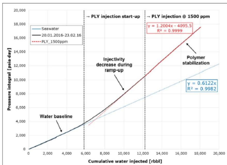
**Figure 2** Hall plot from the polymer injection start-up. A clear change of slope can be observed but with a rapid stabilization and good injectivity (Spagnuolo et al., 2017).
