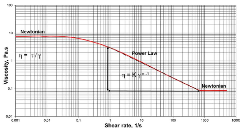
**Figure 4** Typical rheological curve for a polyacrylamide solution. At low end shear rate, two Newtonian plateaus are observed with a conventional rheometer.
