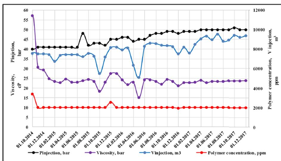
**Figure 3** Evolution of pressure in one injection well for the Kazakh project. A continuous and gentle increase can be observed over 2 years before stabilization (Sagyndikov et al., 2018).
