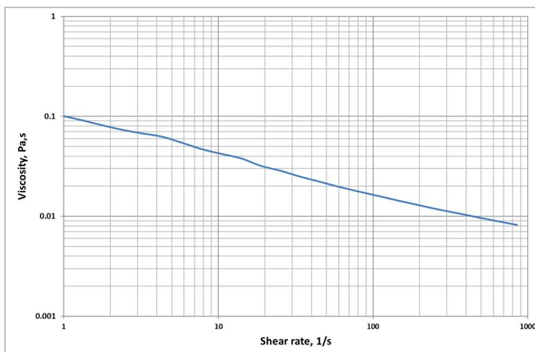
**Figure 5** Flow curve of Flopaam 3630 S in 10 g/L NaCl brine at 25°C. Note the difference between the viscosity at low shear and high shear rate which is 1 order of magnitude in this case.
