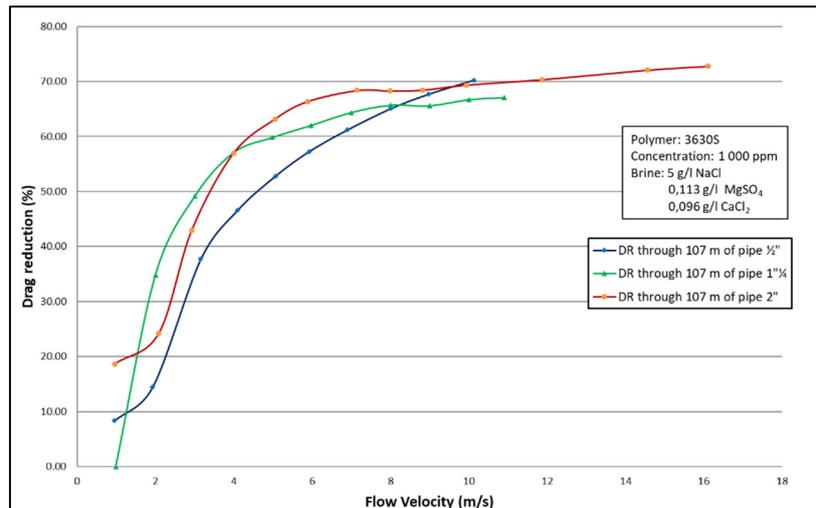
**Figure 7** Drag reduction (%) versus flow velocity through 3 pipes with different diameters (1/2", 1" 1/4 and 2") and a length of 107 meters. Polymer solution: Flopaam 3630S @1000ppm (15cP@7,34s<sup>-1</sup> and 20°C). Drag reduction occurs at velocities above 1 m/s and plateaus between 60% and 70% at high velocity.
