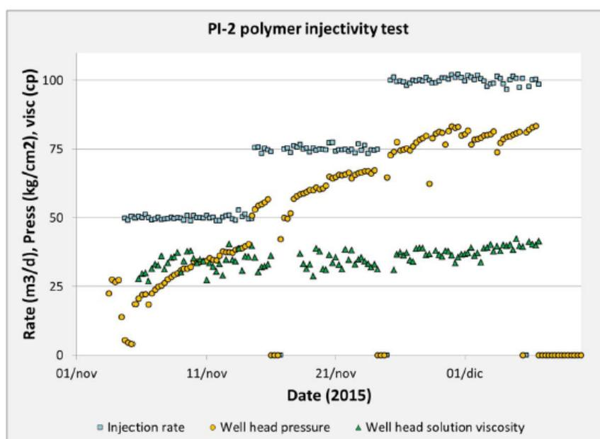
**Figure 1** Graph showing the evolution of pressure during polymer injection as injection rate is varied (Martino et al., 2017).
