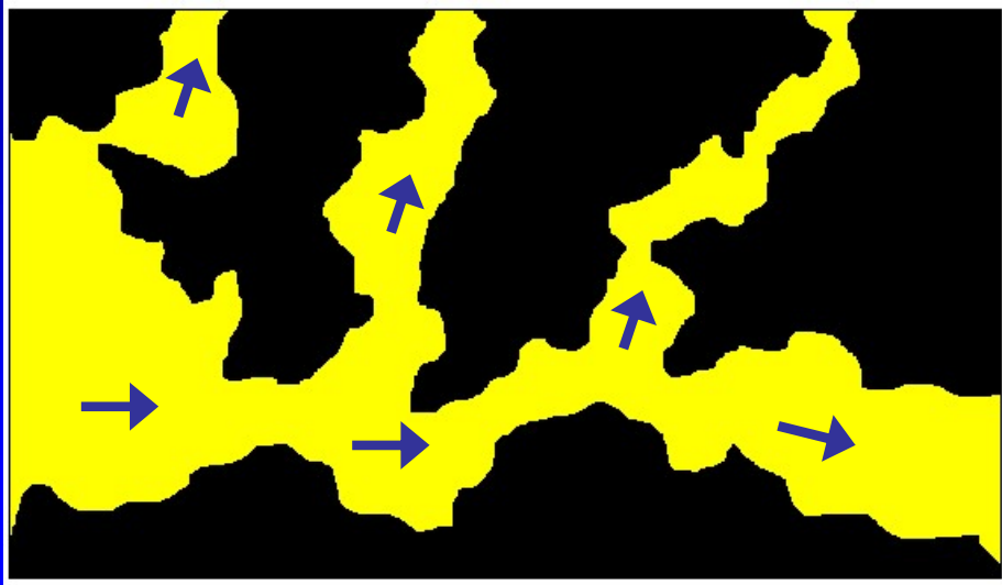
Gelant flows freely like a polymer solution
