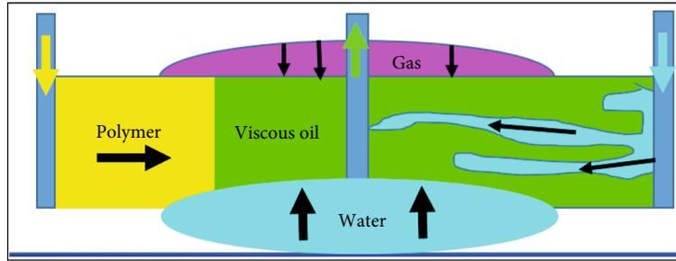
FIGURE 1: Illustration of sources of pressure to push oil toward a production well.
