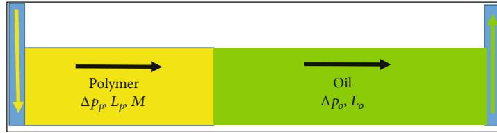
FIGURE 2: Simple linear, piston-like displacement of oil in a single layer.
