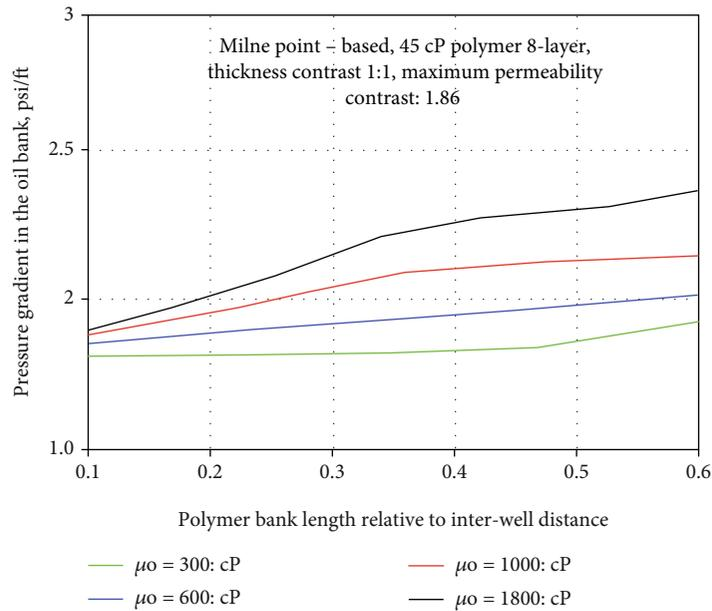
FIGURE 9: Simulation predicted pressure gradients in the oil bank at Milne Point—based (eight-layer).
