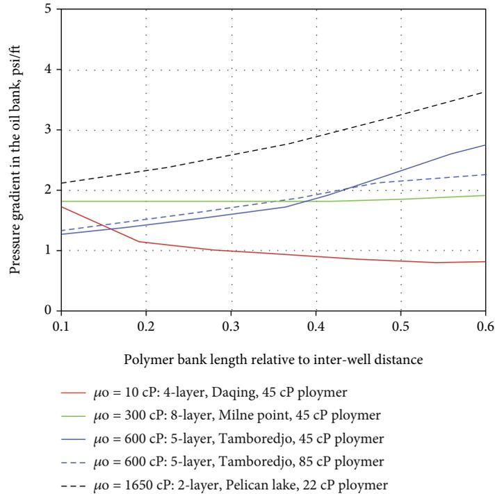
FIGURE 8: Simulation predicted pressure gradients in the oil bank at various oil field conditions.
