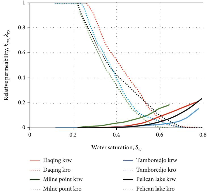
FIGURE 6: Relative permeability curves used in simulations after smoothing.
