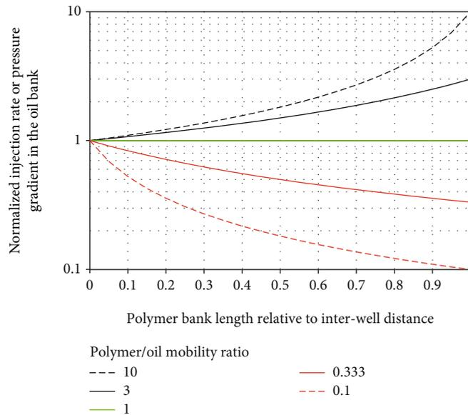
FIGURE 3: Normalized injection rate or pressure gradient in the oil bank versus polymer/oil mobility ratio and polymer bank length.
