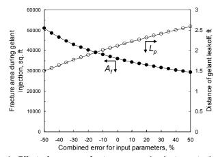
Fig. 1—Effect of errors on fracture area and gelant penetration calculations.
