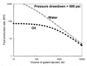
Fig. 5—Production rates versus gelant volume: ⊿p=500 psi.
