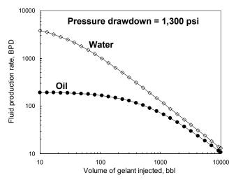
Fig. 4—Production rates versus gelant volume: ∠p=1,300 psi.
