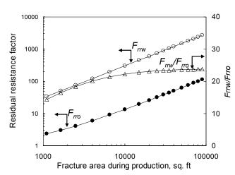
Fig. 2—Sensitivities for calculated *in situ* residual resistance factors.
