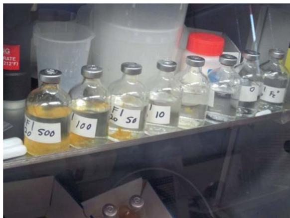
**Fig. 9**—The 2,000-ppm HPAM-ATBS in 2.85%-TDS water with various FeCl<sub>3</sub> levels (0 to 500 ppm), 10-ppb initial O<sub>2</sub>. Day 0.
