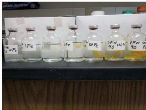
**Fig. 10**—The 2,000-ppm HPAM-ATBS in 11%-TDS brine with various FeCl<sub>3</sub> levels (0 to 500 ppm), 10-ppb initial O<sub>2</sub>. Day 0.
